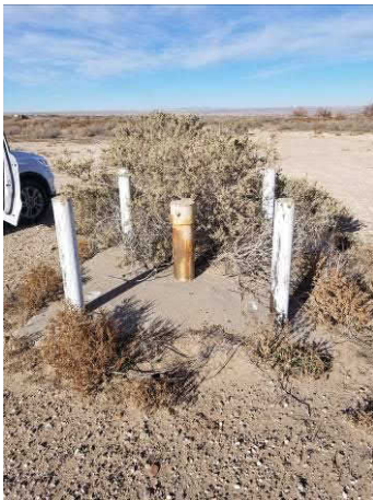
Photo #9 Adjacent: Monitoring well north of the central portion of the site (former landfill monitoring well)
